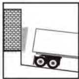
Tapered (incline approach)
