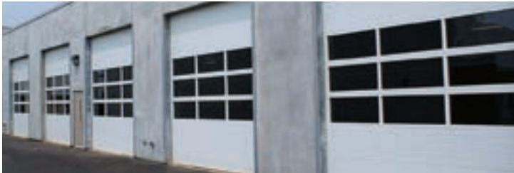
Full-View Aluminum window sections are available for both 2" thick Insulated Sandwich and Ribbed Steel doors for maximum visibility and light.
